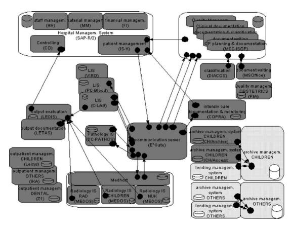
**Fig. 3.** Part of a HIS architecture showing the computer-based application systems, their communication interfaces and communication links between them using the  $3LGM^2$  meta model [19].
